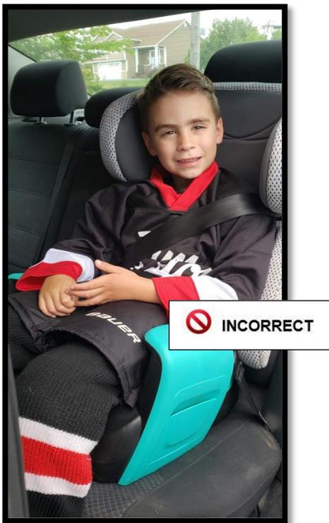
As seen above, wearing padding in a vehicle, will significantly affect seatbelt fit. Shoulder strap is incorrectly sitting too low on the child's arm, and the belt is fitted to hockey gear rather than the child's body.
